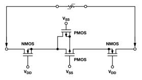
Figure 11. High-voltage fault-protected switch architecture.
