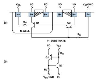
Figure 12. Parasitic SCR structure: a) device b) equivalent circuit.
