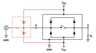
Figure 8. Resistor-diode protection network.
