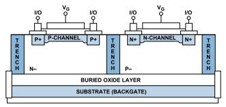
Figure 13. Trench isolation in latch-up prevention.
