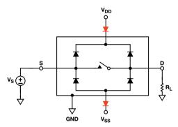
Figure 9. Blocking diodes in series with supplies.
