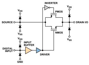
Figure 1. Standard analog switch circuitry.
