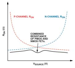
Figure 2. Standard analog switch R<sub>ON</sub> graph.
