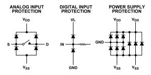
Figure 14. Analog switch ESD protection.
