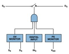
Figure 10. ADG4612/ADG4613 switch architecture.
